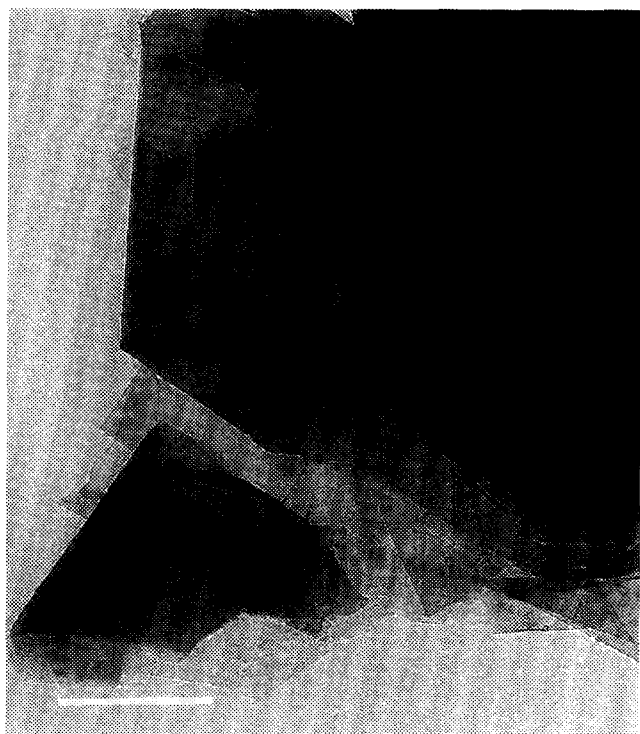
Figure 1 Transmission electron micrograph of sPS crystals formed from dilute solution in ethylbenzene. The bar represents 0.40 \mu\text{m}
